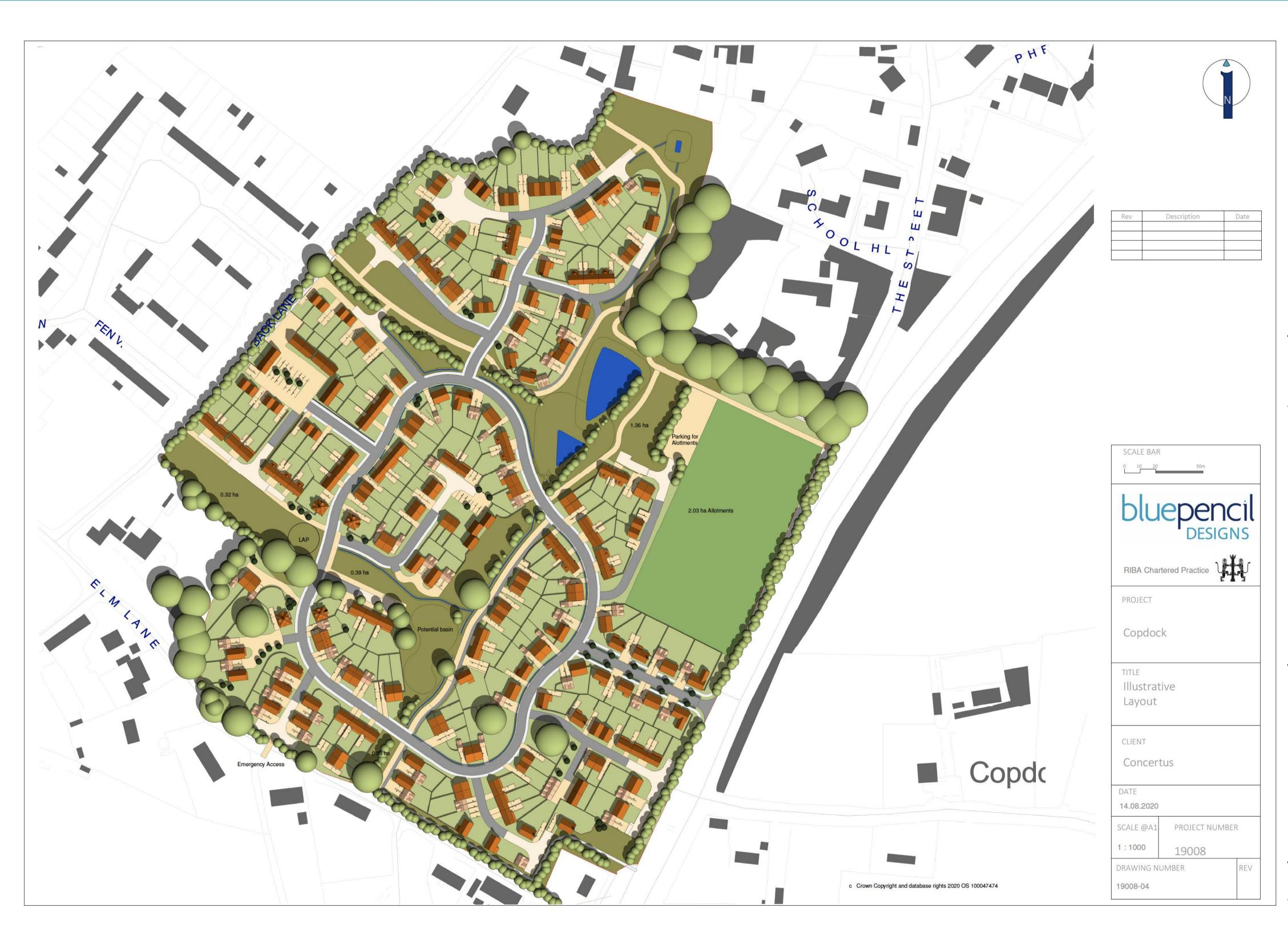
It is proposed that the site will be accessed by a single junction positioned on the south-east corner of the site. More specifically, a priority junction on London Road with a right turn lane will be created.
